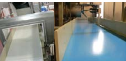
Replacing interlocking belts with smooth belts has saved labour and cleaning time and has improved food safety.
